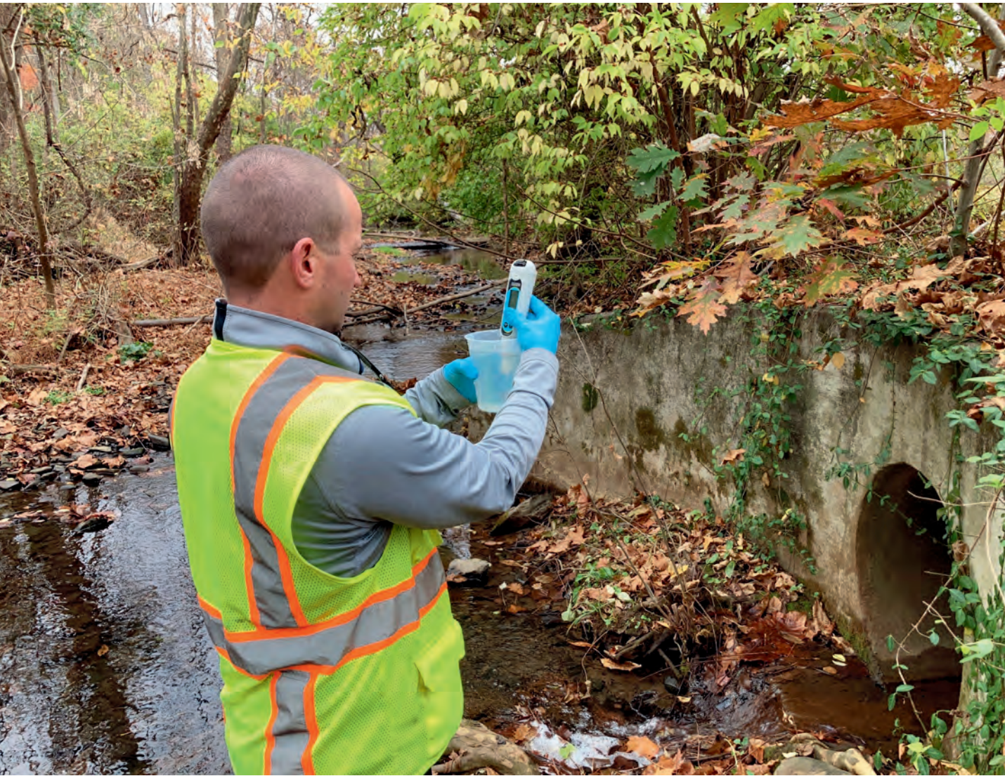
Roanoke County’s stormwater inspector, Daniel Hood, evaluates a water sample from an active discharge at an outfall pipe. His goal is to determine if there are any obvious pollutants in the discharge, such as sediment, detergent, oil, or sewage. Should an illicit discharge be likely, he will arrange for additional testing at a local environmental laboratory. Once an illicit discharge is confirmed, he will locate the source and work with the responsible party to eliminate the illicit discharge.
